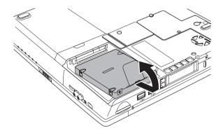
Figure 8-17 Removing the HDD pack
